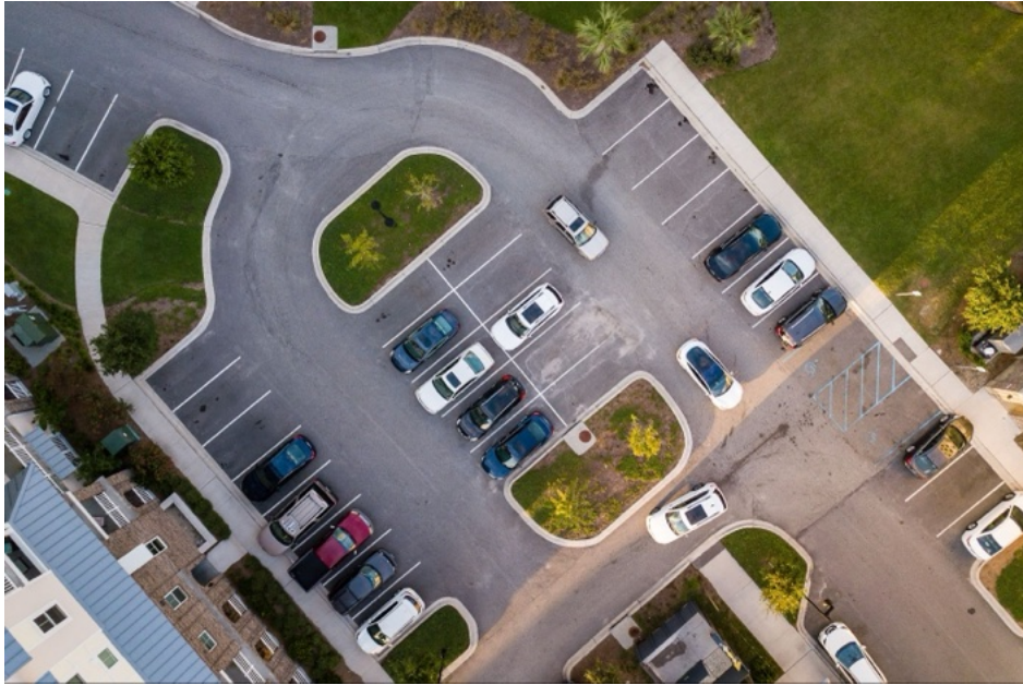
Standard 90-degree parking with 24' drive aisle, consistent with Avian Commons and Berkeley County standards.
