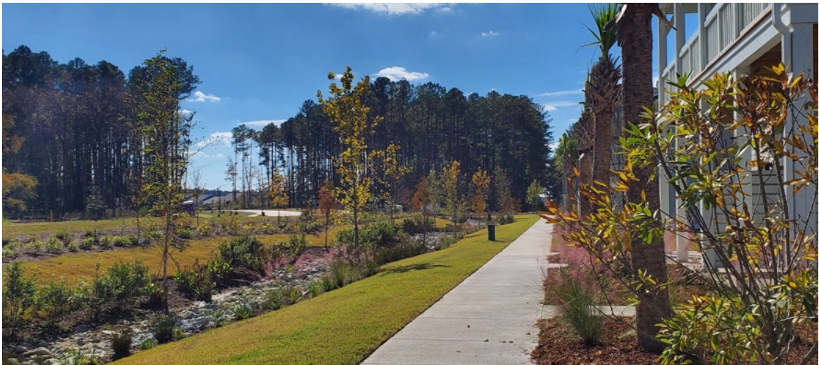
This planted bioswale filters runoff, reduces flooding, and adds ecological and aesthetic value through strategic vegetation.
